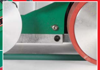
Air partition for homogenous welding seam
